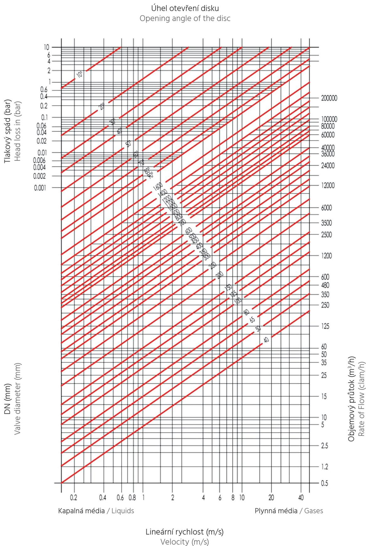
**KOEFICIENT PRŮTOKU  $K_v$  ( $m^3/h$ ) V ZÁVISLOSTI NA ÚHLU OTEVŘENÍ KLAPKY (DISKU)**
