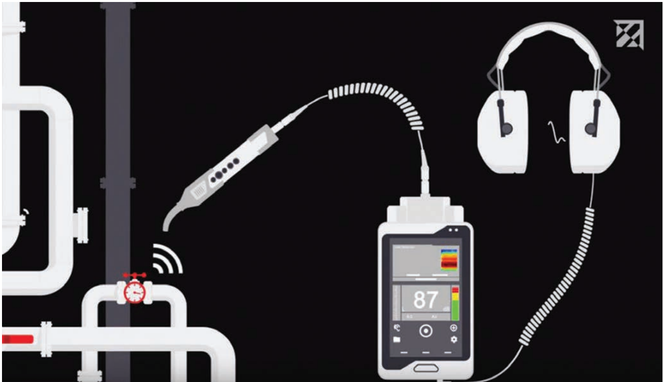
Fig. 10 - Ultrasonic leak detection principle
