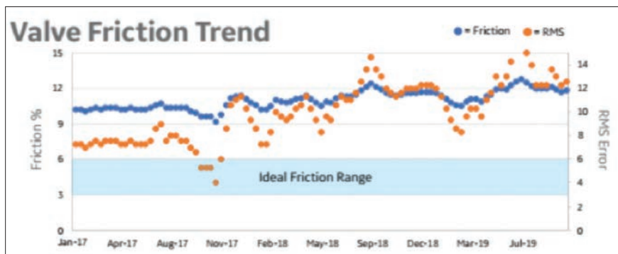
Fig. 6 - Graph of friction in packing
